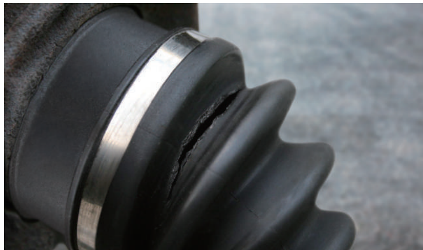
Cracked C.V. Boot
